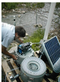
Fig. 3a. Servicing “R 2 D 2 ” the Teledyne ISCO automated water sampler located at the Rt 38A site. It collected 1-liter of water every 8-hrs and was serviced weekly.
